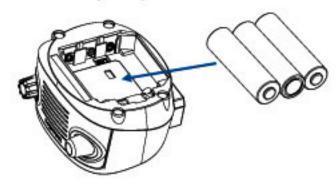
Step3: Reinstall the battery cover and screws. After the batteries are inserted, the GREEN Power LED will automatically light and flash.
