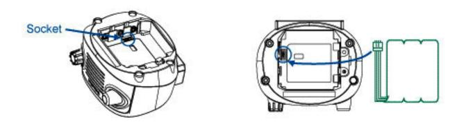
Step3: Reinstall the battery cover and screws, and then plug the wall transformer in to an AC receptacle if needed. After the batteries are inserted, the GREEN Power LED will automatically light.
