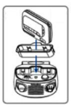
Before inserting the right pager type dock adapter, please be sure to remove the screws which are fitted inside the socket.
