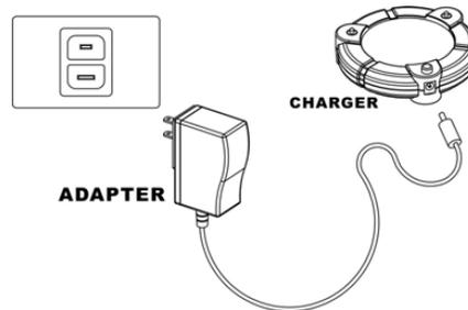
**Step 2:** When the charger is powered, the charger power LED will illuminate to show it is on.
