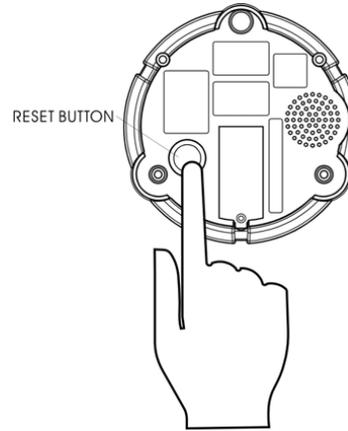
To stop the audible and vibrate alert, press **Reset button**.
